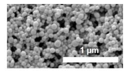
Fig. 1. SEM micrograph of HA Nano at 37 °C.
