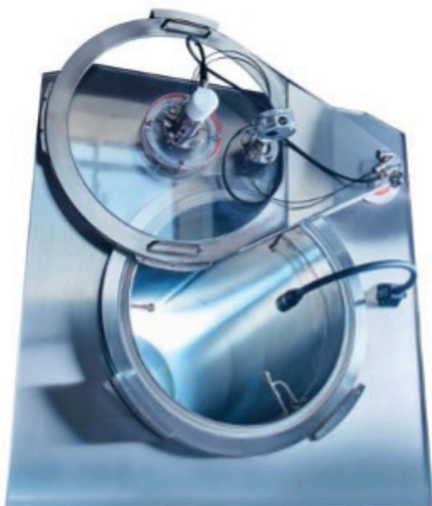
Fig.2.2.4: Top Lid with Spray Nozzle of the Spray-Freeze Chamber. (Courtesy Meridion)
