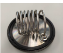
Fig. 1: Disassembled small cooling coil with 7 coil windings
